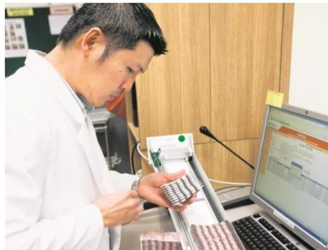
3. Medicines are packed in cartridges which are slotted into the picking robots.
