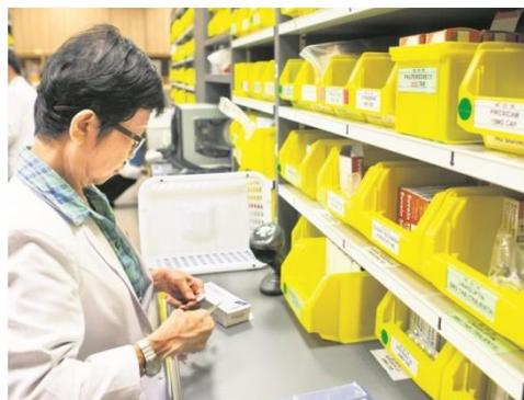
5. For drugs that need manual picking – when the drug's barcode is scanned, the LED on the drug bin lights up, guiding staff to the right drug.
