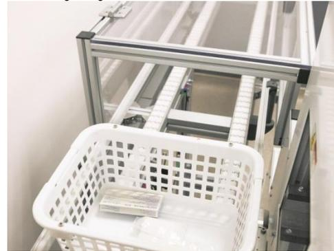
2. The baskets travel on a conveyor where RFID readers provide real-time tracking of the drugs.
